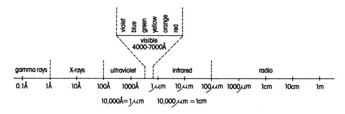
Schematic diagram of the electromagnetic spectrum, ranging from the shortest wavelengths (gamma rays) to the longest (radio waves). The wavelength of light is measured in Ångstroms (Å), micrometers (µm), centimeters (cm) and meters (m).
